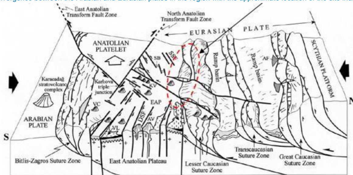
Figure 11.2: Block diagram depicting compressional and tensional neotectonic structures resulting from north-south convergence between the Arabian and Eurasian plates in the region with the approximate location of the site indicated.
