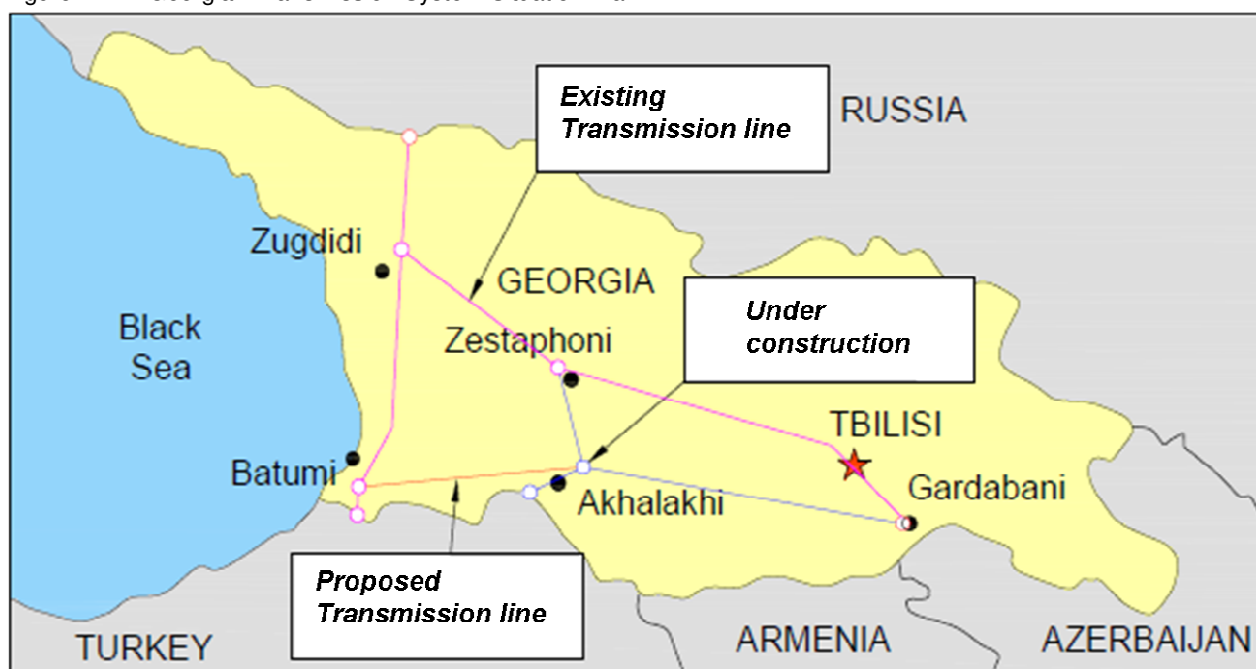
Figure 2.4: Georgian Transmission System Situation Plan
