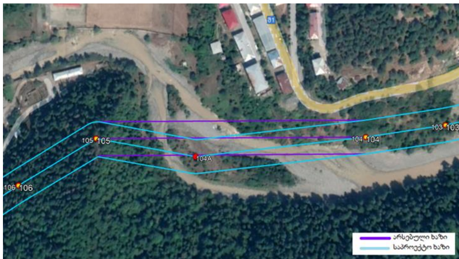
Figure 4: Existing and proposed sections of the 35 kV Skhalta-Shuakhevi OTL (between towers NN 103 and 106)
