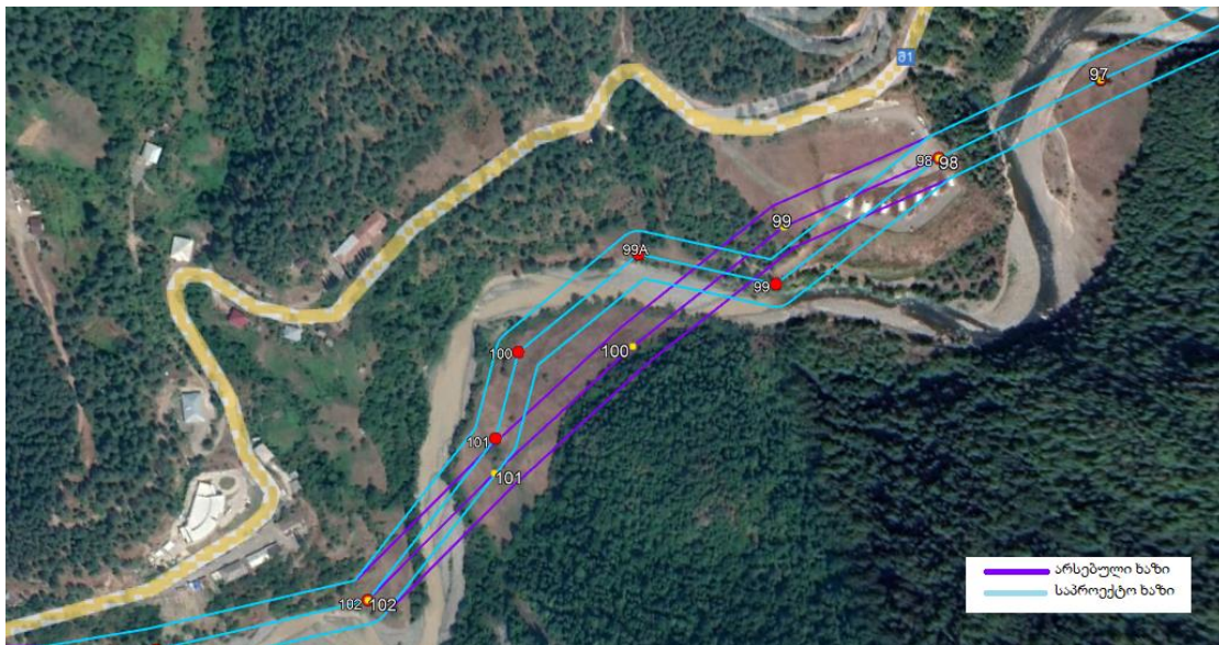
Figure 2.: Existing and proposed design route of the 35 kV Skhalta - Shuakhevi OTL (between towers NN 97 and 102)
